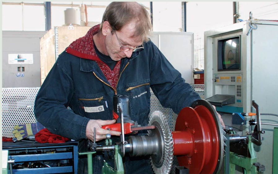
Turbo Engineering's balancing bay at its Rotterdam centre
